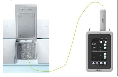
Place the cable of LEO's probe so that the tip of the sensor touches the bottom of the dish.
